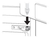
2 Fit the hinge ① over the hinge lever latch ② and slot it into place. Rotate the lever ③ counterclockwise to secure the hinge.
