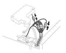
**4** Push the water supply tube into the hole on the top case and pull it through the backplate.
