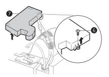
Remove the cover and pull out the tube <sup>(3)</sup>.Disconnect all wire harnesses <sup>(9)</sup>. Unscrew the ground wire <sup>(10)</sup>.
