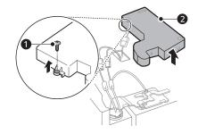
2 Detach all the wire harnesses ③. Unscrew the ground wire ④. Remove the cover.
