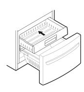
**5** Replace the ice bin in the drawer. Insert the Durabase basket in the rail assembly.
