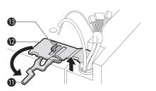
**5** Lift the door from the middle hinge pin and remove the door.
