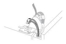
5 Hold the water supply connection and gently push in the collet <sup>(1)</sup> to connect the water supply line as shown. Insert the tube at least 5/8 inch (15 mm) into the connector. Insert the clip on the joint to fasten the tube in place.
