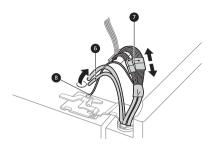
**3** Rotate the hinge lever **9** counterclockwise. Lift the top hinge **10** free of the hinge lever latch **10**.
