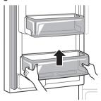
To replace the bin, slide it in above the desired support and push down until it snaps into place.
