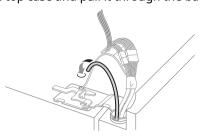
Hold the water supply connection and gently push in the collet 4 to connect the water supply line as shown. Insert the tube at least 5/8 inch (15 mm) into the connector. Insert the clip on the joint to fasten the tube in place.
