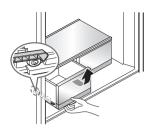
Lift the front of the cover with one hand and support underneath the cover with the other hand.
