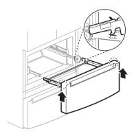
3 Lower the door into its final position and insert the screws in the rails on both sides.
