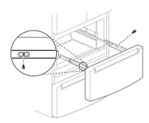
**3** Grip both sides of the drawer and pull it up to remove it from the rails.
