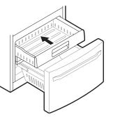
**5** Replace the ice bin(s) in the drawer. Insert the Durabase basket in the rail assembly.
