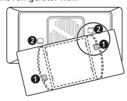
**5** Rotate the air filter cover clockwise until the hooks engage and the cover locks in place.
