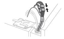
**4** Push the water supply lines into the hole on the top case and pull them through the backplate.
