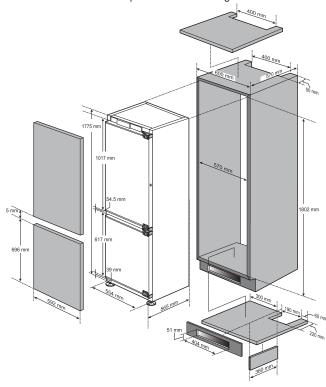
• The dimension of the door panels changes if there is a change of cabinet material thickness.
