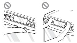
• Do not push or pull the range by grabbing the open oven door or cooktop only. Doing so can result in serious damage to the range.
