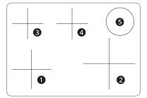
Induction Left Front Cooking Element: 8", 2100 W / 3200 W (240 V)
