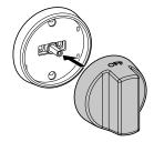
Push the knob onto the shaft as far as possible so it fits snugly.
