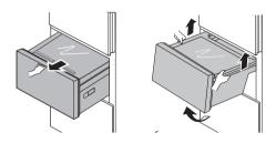
To reassemble the drawer, align it with the rails and insert it until it stops, lift it to clear the safety rail stops and push it in completely.
