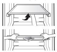
To remove the pantry drawer, lift it slightly and pull it out. To assemble the drawer, align it with the grooves at either side and slide it in. (Empty the drawer before removing or assembling it.)
