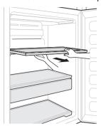
2 Press on the hook inside the top compartment, and then take out the Fresh Air Filter.
