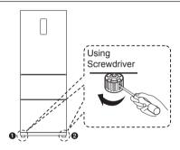
To level the refrigerator, use a screwdriver to turn the leveling feet until they are in firm contact with the floor. The front of the refrigerator can be slightly higher than the rear to make shutting the doors easier.
