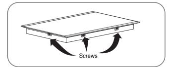
2 Carefully lower the cooktop into the counter- top cutout, making sure not to trap any wires. NOTE: Do not use caulking compound. The cooktop must be removable, should service be required.
