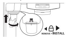
After the water filter is replaced, dispense 2.5 gallons of water (flush for approximately 5 minutes) to remove trapped air and contaminants from the system.
