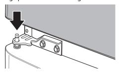
Place the top hinge on top of the freezer door and line up the top hinge with the holes on top of the refrigerator. Use the three bolts to attach the hinge.
