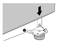
2 Place the middle hinge pin 2 inside the hinge pin sleeve 3 on the top of the refrigerator door.
