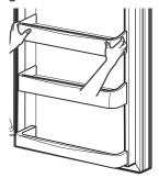
To assemble the bin, slide it in above the desired support and push down until it snaps into place.
