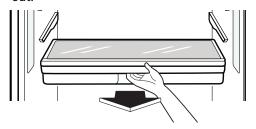
To assemble, slide the drawer back all the way past the drawer stop.
