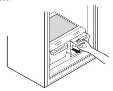
To reassemble, slightly tilt up the front of the crisper, insert it into the frame, and push it back into place.
