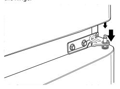
**3** Carefully snap the top hinge cover back into place over the hinge.
