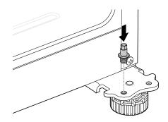
Using a 3/8 in. socket wrench with a 2-inch extension, loosen the 2 bolts on the bottom hinge bracket. Use a Phillips screwdriver to loosen the screw.
