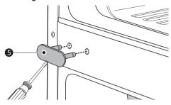
Remove the decorative screw 6 located on the housing between the freezer and refrigerator doors. (You will need this hole for the middle hinge bracket.)
