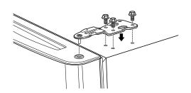
Place the top hinge on top of the freezer door and line up the hinge with the holes on top of the refrigerator. Use the three bolts to fasten the hinge.
