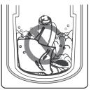
• Do not load bulky items such as pet beds that are too large or stiff to move easily around the agitator. Impeding the motion of the drum or agitator could cause damage to the items or the washer.
