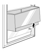
To reassemble, slightly tilt up the front, insert the drawer into the frame and push it back into place.
