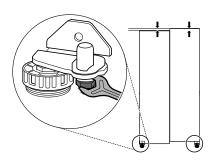
Open the door and use the wrench 10 to loosen the keeper nut by turning it to the left.
