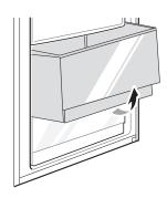
2 To reassemble, slightly tilt up the front, insert the drawer into the frame and push it back into place.
