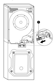
**2** Connect the drain hose of the dryer and secure the hose clamp.
