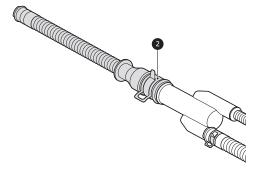
Securely connect the short drain hose to a floor drain or standpipe. When connecting to a waste spigot, use a band clamp 3 on the end of the short drain hose.
