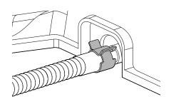
Screw in the band to secure the drain hose of the dryer onto the stacking bracket.
