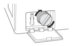
Close the drain pump filter cover.
