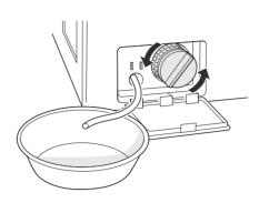
**5** Clean the pump filter and opening.
