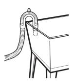
**3** Use the provided tie strap to secure the drain hose in place.
