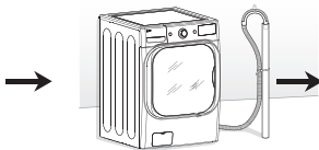
Connecting the drain line
