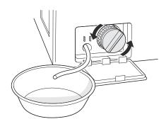
**5** Clean the pump filter and opening.
