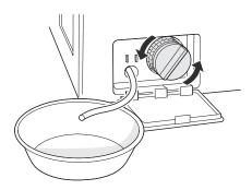
**5** Clean the pump filter and opening.
