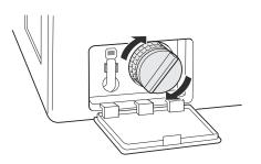
**8** Close the drain pump filter cover.
