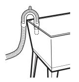
**3** Use the provided tie strap to secure the drain hose in place.
