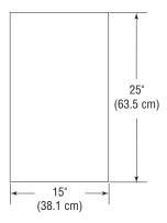
Panel should be 1/2" (13 mm) min. thickness
