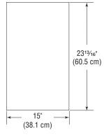
Panel should be 1/2" to 5/8" (13 to 16 mm) thick. NOTE: A thicker panel may need rounded front corners and a cutout for access to the handle.
