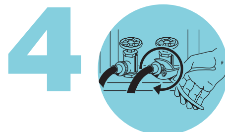
Connect to cold water supply. For more information, see Installation Instructions section of Use and Care Guide.
