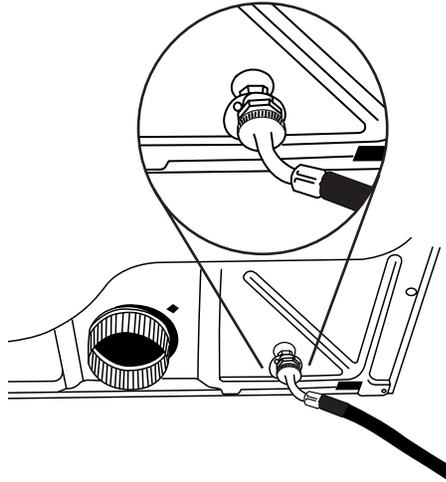
**NOTE:** Do not overtighten. Damage to the coupling can result.
