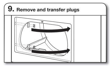
Remove the four screws that attach two plugs on the left side. Transfer plugs to opposite side using the same four screws.
