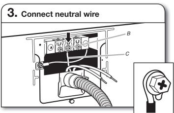
Place hooked end of neutral wire (white or center) (C) of direct wire cable under center terminal block screw (B). Squeeze hooked end together. Tighten screw.
