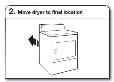
Move dryer to final location. Avoid crushing or kinking vent. After dryer is in place, remove corner posts and cardboard from under the dryer.
