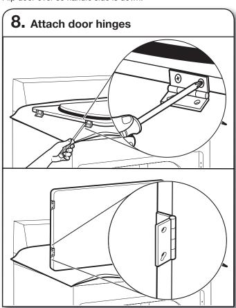
Reattach door hinges to dryer door so that the larger hole is at the bottom of the hinge.
