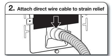
Put direct wire cable through the strain relief. The strain relief should have a tight fit with the dryer cabinet and be in a horizontal position. Tighten strain relief screw against the direct wire cable.
