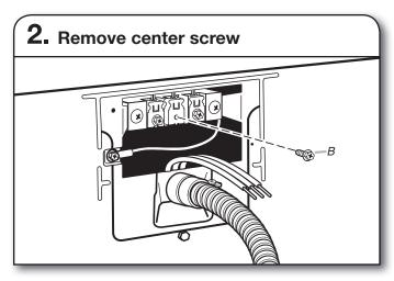
Remove center terminal block screw (B).
