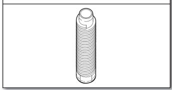
Using a wrench and tape measure, screw legs into leg holes until bottom of foot is approximately  $1\frac{1}{2}$ " (38 mm) from bottom of dryer.
