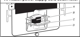
Remove the screws from a 3/4" (19 mm) UL Listed strain relief. Put the tabs of the two clamp sections (C) into the hole below the terminal block opening (B) so that one tab is pointing up (A) and the other is pointing down (D), and hold in place. Tighten strain relief screws just enough to hold the two clamp sections (C) together.
