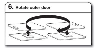
Rotate outer door 180° and set it back down on inner door. Be certain to keep cardboard spacer centered between doors. Reattach outer door panel to inner door panel so handle is on the side where hinges were just removed. Insert six door screws.
