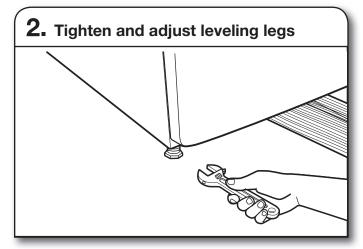
If dryer is not level, prop up using a wood block, use wrench to adjust legs up or down, and check again for levelness. Once dryer is level, make sure all four legs are snug against the floor before tightening them.
