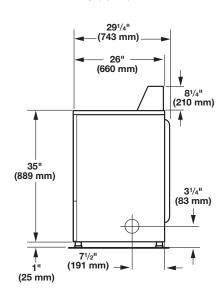
Most installations require a minimum 5½" (140 mm) clearance behind the dryer for the exhaust vent with elbow. See "Venting Requirements."
