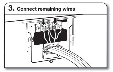
Place hooked ends of remaining wires under outer terminal block screws (hooks facing right). Tighten screws.
