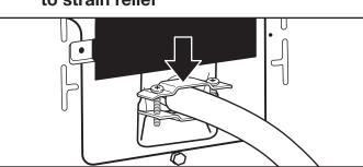
Put power supply cord through the strain relief. Be sure that the wire insulation on the power supply cord is inside the strain relief. The strain relief should have a tight fit with the dryer cabinet and be in a horizontal position. Do not further tighten strain relief screws at this point.
