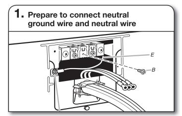
Remove center terminal block screw (B). Remove neutral ground wire (E) from external ground conductor screw (A).
