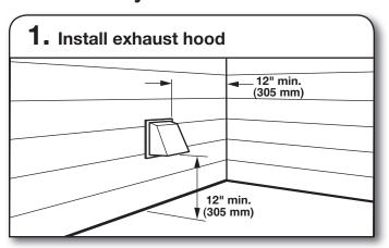
Install exhaust hood and use caulking compound to seal exterior wall opening around exhaust hood.
