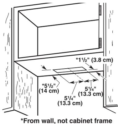
To make a circular vent opening on the underside of the cabinet top:
