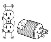
The Drying Center gas model is designed to operate on a 120-volt/20-amp circuit, using an electrical plug and outlet similar to those shown. If your laundry room doesn't have this type of outlet, contact an electrician who can install a proper outlet designed to carry the necessary amperage. The laundry outlet must be less than 6 feet from the washer/gas dryer.
