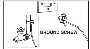
**NEVER CONNECT GROUND WIRE TO PLASTIC PLUMBING LINES, GAS LINES OR HOT WATER PIPES.**
