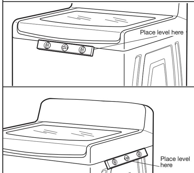
Check the levelness of the washer. First, place a level on the lid near the console. Then place the level on the side of the washer in the crease between the top of the washer and the cabinet.
