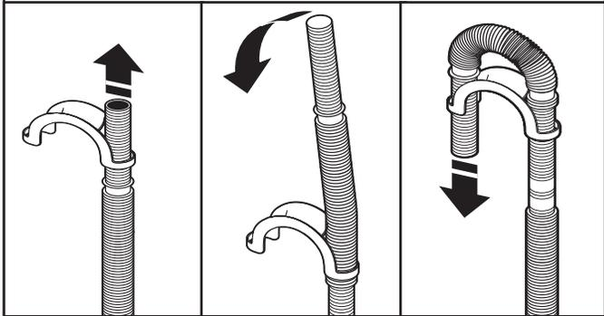
For a laundry tub or standpipe drain, connect the drain hose form. For a floor drain, do not install drain hose form. You may need alternate parts with separate directions. See “Tools and Parts” to determine what you may need.
