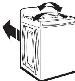
Move the washer to its final location. Rock the washer back and forth to check whether all four feet are stable and in firm contact with the floor. If the washer rocks, minor adjustments may be needed to level the washer on your floor.
