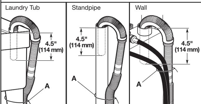
Secure drain hose to laundry tub leg, drain standpipe, or inlet hoses for wall standpipe with cable tie (A). This will help reduce the chance of drain water splashing on the floor.
