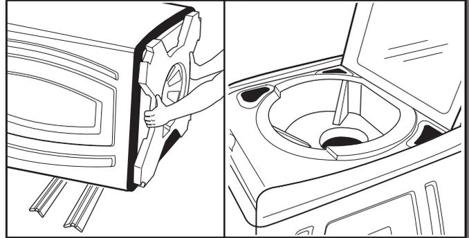
Place cardboard supports from shipping carton on floor behind washer for support. Secure the lid with tape. Using two or more people, tip the washer onto its back and place on cardboard supports. Remove foam shipping base. Then, set washer back upright, and remove the tape from the lid so that you can open the lid and remove the foam packing ring from the washer tub.
