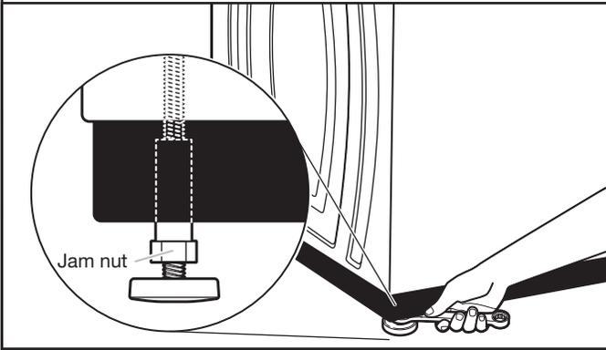
If washer is not level, use a 9/16" or 14 mm open-end or adjustable wrench to turn jam nuts clockwise on feet until they are about 1/2" (13 mm) from the washer cabinet. Then turn the leveling foot clockwise to lower the washer or counterclockwise to raise the washer. Recheck levelness of washer and repeat as needed.
