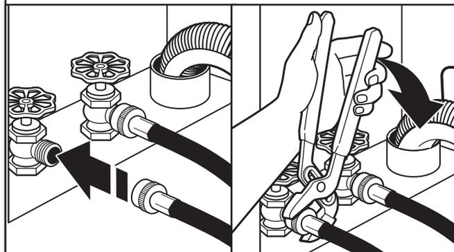
Make sure the washer basket is empty. Attach the hose labeled hot to hot water faucet. Screw on coupling by hand until it is seated on washer. Use pliers to tighten couplings an additional two-thirds turn. Repeat this step with the hose labeled cold for the cold water faucet. Both hoses must be connected for washer to work properly.
