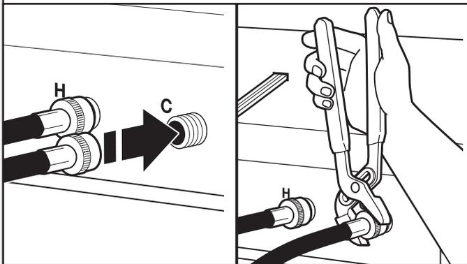
Attach hot water hose to hot water inlet valve. Screw coupling by hand until it is snug. Use pliers to tighten couplings an additional two-thirds turn. Repeat with cold water inlet valve. Both hoses must be connected for washer to work properly.
