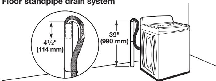
Minimum diameter for a standpipe drain: 2" (51 mm). Minimum carry-away capacity: 17 gal. (64 L) per minute. Top of standpipe must be at least 39" (990 mm) high; install no higher than 96" (2.4 m) from bottom of washer. If you must install higher than 96" (2.4 m), you will need a sump pump system.
