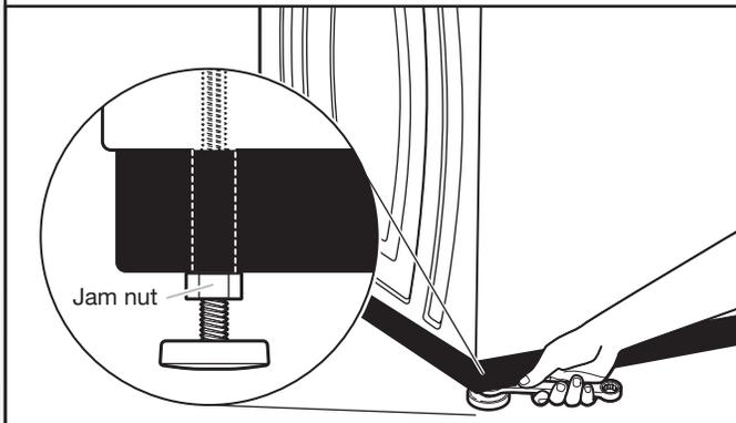
When washer is level, use a 9/16" or 14 mm open-end or adjustable wrench to turn jam nuts counterclockwise on leveling feet tightly against washer cabinet.
