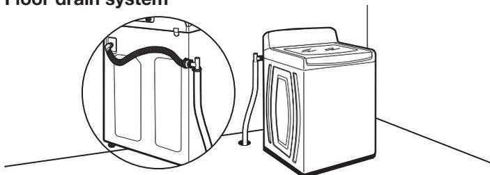
Floor drain system requires a Siphon Break Kit (Part Number 285834), 2 Connector Kits (Part Number 285835), and an Extension Drain Hose (Part Number 285863) that may be purchased separately. To order, please see toll-free phone numbers in your "Use and Care Guide." Minimum siphon break: 28" (710 mm) from bottom of washer. (Additional hoses may be needed.)
