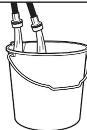
Run water for a few seconds through hoses into a laundry tub, drainpipe, or bucket to avoid clogs. Water should run until clear. Check the temperature of the water to make sure that the hot water hose is connected to the hot water faucet and the cold water hose is connected to the cold water faucet.
