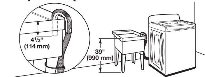
Minimum capacity: 20 gal. (76 L). Top of laundry tub must be at least 39" (990 mm) above floor; install no higher than 96" (2.4 m) from bottom of washer.
