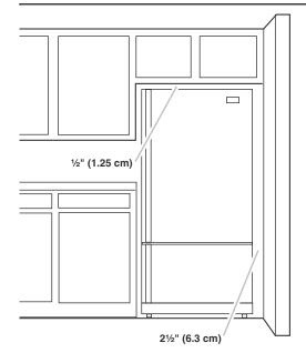
To ensure proper ventilation for your refrigerator, allow for a ½" (1.25 cm) space at the top and behind the refrigerator. If your refrigerator has an ice maker, allow extra space at the back for the water line connections. When installing your refrigerator next to a fixed wall, leave 2½" (6.3 cm) minimum on the hinge side (some models require more) to allow for the door to swing open.
