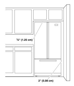
To ensure proper ventilation for your refrigerator, allow for a ½" (1.25 cm) of space on each side and at the top. Allow for a 1" (2.54 cm) space behind the refrigerator. If your refrigerator has an ice maker, allow extra space at the back for the water line connections. When installing your refrigerator next to a fixed wall, leave a 2" (5.08 cm) minimum space between the refrigerator and wall to allow the door to swing open.
