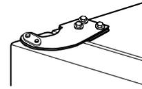
4. Align the doors so that the bottom of the freezer door aligns evenly with the top of the refrigerator door. Tighten all screws.
