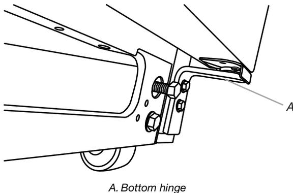
3. Measure the distance from the bottom of the refrigerator door to the floor. The distance should be approximately 3 1/2" (88 mm).
