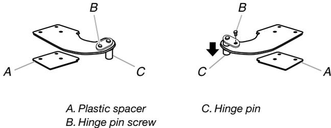
3. Fasten the top hinge to the opposite side of the cabinet, inserting the screws only halfway, so you will be able to replace and align the freezer door later.
