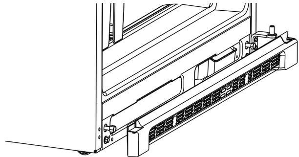
8. Using a hex-head socket wrench, remove the two  $\frac{5}{16}$ " hex-head hinge screws attaching the bottom hinge to the cabinet and remove the hinge from the bottom of the refrigerator door.
