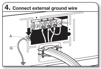
Connect a separate copper ground wire (G) under the green external ground conductor screw (A) to an adequate ground. Finally, reinsert tab of terminal block cover into slot of dryer rear panel. Secure cover with hold-down screw. Now, go to Venting Requirements.
