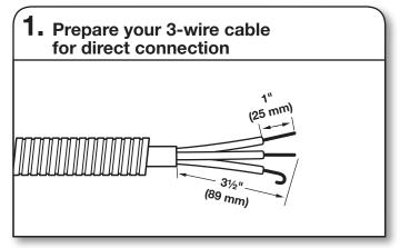
Direct wire cable must have 5 ft. (1.52 m) of extra length so dryer may be moved if needed.
