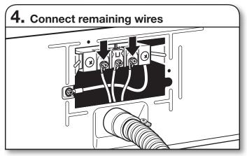
Place hooked ends of remaining direct wire cable wires under outer terminal block screws (hooks facing right). Squeeze hooked ends together and tighten screws. Finally, reinsert tab of terminal block cover into slot of dryer rear panel. Secure cover with hold-down screw. Now, go to Venting Requirements.
