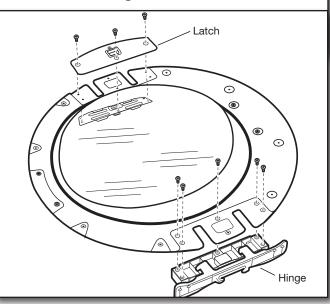
Using a  $Torx^{\circ}$  T25 screwdriver, remove the 3 Torx screws securing the latch plate and latch backing plate and the 5 screws holding the hinge assembly in place.
