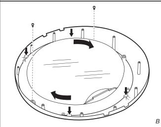
With the edge with 2 notches at the top, align the notches on the outer window assembly with the tabs on the trim ring and lower into place as shown in figure A.
