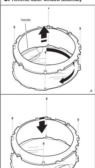
Using a Phillips screwdriver, remove the 4 screws from the outer window retainer and lift off the trim ring off the window (A). Rotate trim ring 180° and secure with the 4 screws removed earlier (B).
