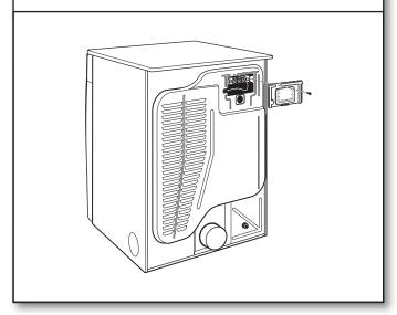
Remove hold-down screw and terminal block cover.
