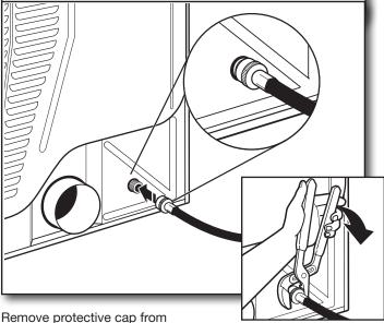
water inlet valve. Attach other end of long hose to fill valve at bottom of dryer back panel. Screw on coupling by hand until it is seated on fill valve connector. Using pliers, tighten the couplings an additional two-thirds turn.
