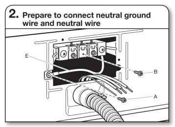
Remove center terminal block screw (B). Remove neutral ground wire (E) from green external ground conductor screw (A).
