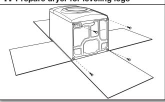
To avoid damaging floor, use a large flat piece of cardboard from dryer carton; place under entire back edge of dryer. Firmly grasp dryer body (not console panel) and gently lay dryer down on cardboard.
