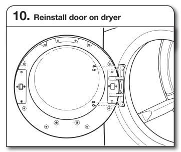
Using a Torx® T25 screwdriver, remove the 4 screws on the dryer. Insert the tabs on the hinge into the mounting slot and slide down to engage the top tab. Secure in place with the 4 Torx® T25 screws removed earlier.
