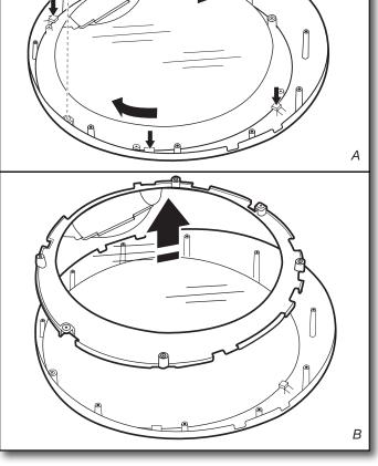
Using a Phillips screwdriver, remove the 2 screws from the outer window retainer and rotate the outer window assembly clockwise until the square notches line up with the 4 tabs on the trim ring indicated with arrows in the figure A above. Then lift out the outer window and retainer up and off the trim ring and set aside (B).
