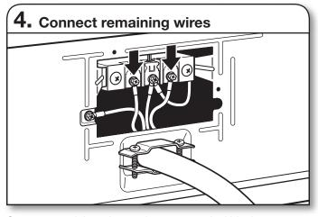
Connect remaining wires under outer terminal block screws. Tighten screws. Finally, reinsert tab of terminal block cover into slot of dryer rear panel. Secure cover with hold-down screw. Now, go to Venting Requirements.
