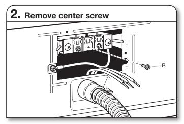
Remove center terminal block screw (B).
