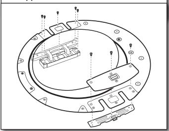
Using a Torx® T25 screwdriver, reinstall the latch plate, latch backing plate, and hinge assembly on the opposite sides from which they were removed.
