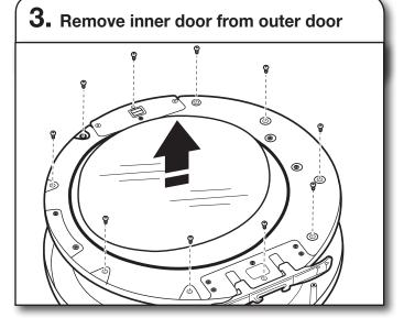
Position the door with the inside of the door facing up. Using a Phillips screwdriver, remove the 10 screws securing the inner door to the outer door. Lift off the inner door and set aside.
