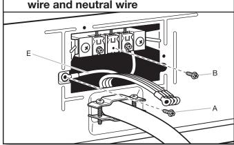
Remove center, silver-colored terminal block screw (B). Remove neutral ground wire (E) from green external ground conductor screw (A).
