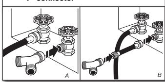
If space permits, attach the female end of the "Y" connector to the cold water faucet. See figure A.
