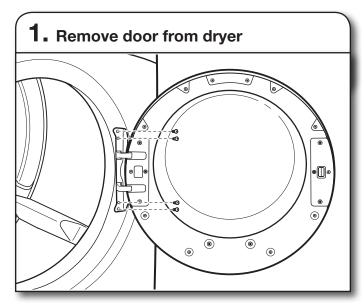
**IMPORTANT:** If the protective film has not yet been removed from the dryer, peel the film from the dryer door before proceeding.
