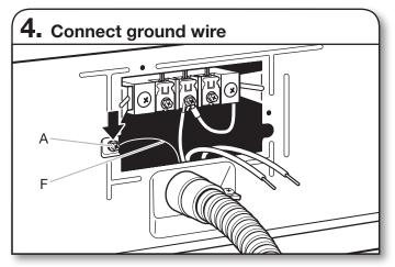
Connect ground wire (green or bare) (F) of direct wire cable under green external ground conductor screw (A). Tighten screw.
