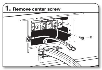
Remove center terminal block screw (B).
