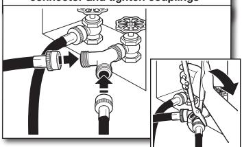
One end of the long hose has a wire mesh strainer inside the coupling. Attach this end to the "Y" connector. Attach washer cold inlet hose to other side of "Y" connector. Screw on coupling by hand until it is seated on connector. Using pliers, tighten the couplings an additional two-thirds turn.
