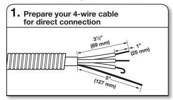
Direct wire cable must have 5 ft. (1.52 m) of extra length so dryer may be moved if needed.
