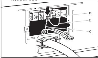
Connect neutral ground wire (E) and neutral wire (white or center) (C) of power supply cord under center terminal block screw (B). Tighten screw.
