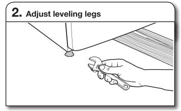
If dryer is not level, prop up using a wood block, use wrench to adjust legs up or down, and check again for levelness. Once dryer is level, make sure all four legs are snug against the floor and dryer does not rock.
