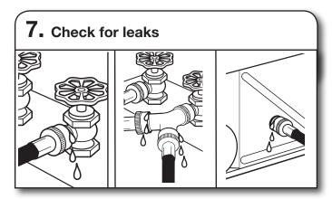
Check for leaks around "Y" connector, faucet, and hoses.
