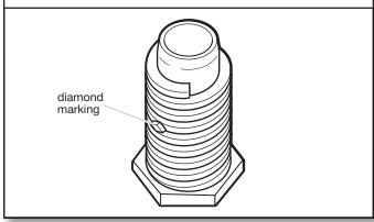
Examine leveling legs, find diamond marking. Screw legs into leg holes by hand, use a wrench to finish turning legs until diamond marking is no longer visible.
