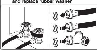
Turn cold water faucet off and remove washer inlet hose.
