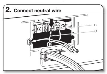
Connect neutral wire (white or center) (C) of power supply cord under center terminal block screw (B). Tighten screw.
