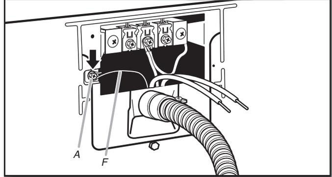
Connect ground wire (green or bare) (F) of direct wire cable to external ground conductor screw (A). Tighten screw.
