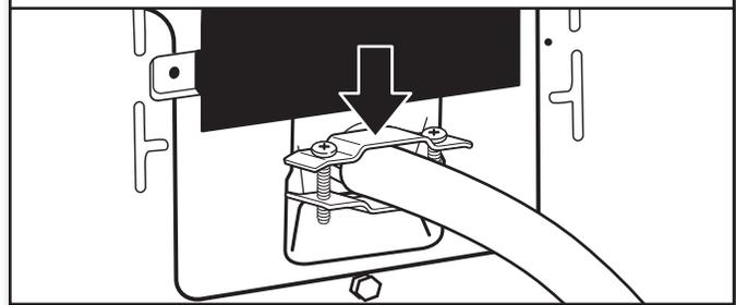
Put power supply cord through the strain relief. Be sure that the wire insulation on the power supply cord is inside the strain relief. The strain relief should have a tight fit with the dryer cabinet and be in a horizontal position. Do not further tighten strain relief screws at this point.
