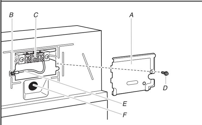
Before you start, disconnect power. Remove hold-down screw (D) and terminal block cover (A).
