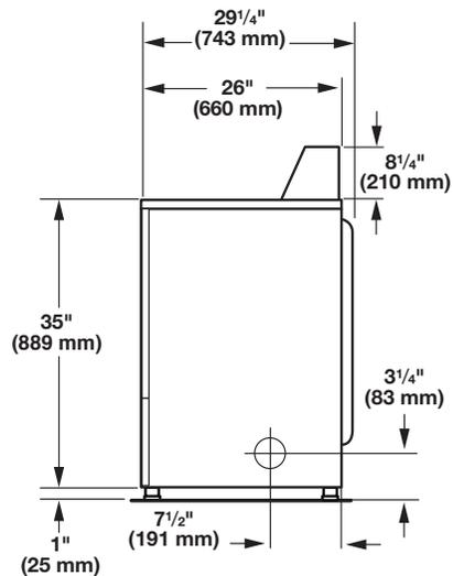
Most installations require a minimum 5 1/2" (140 mm) clearance behind the dryer for the exhaust vent with elbow. See "Venting Requirements."
