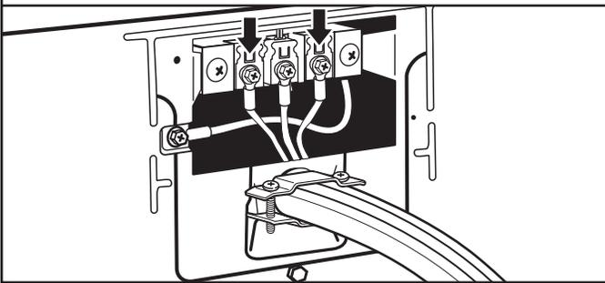
Connect remaining wires to outer terminal block screws. Tighten screws. Finally, reinsert tab of terminal block cover into slot of dryer rear panel. Secure cover with hold-down screw. Now, go to "Venting Requirements."
