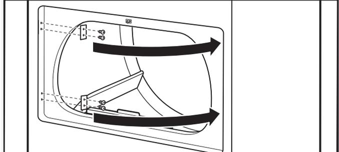
Remove the four screws that attach two plugs on the left side. Transfer plugs to opposite side using the same four screws.
