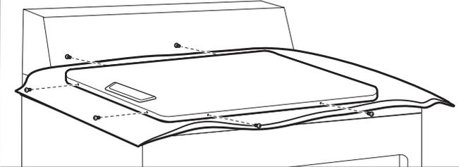
Remove screws at top, bottom, and side of door (six screws). Keep door screws separate from hinge screws as they are different sizes. Holding door over towel on dryer, grasp sides of outer door and lift to separate it from inner door.
