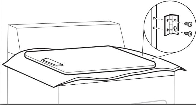
Remove screws attaching hinges to door.
