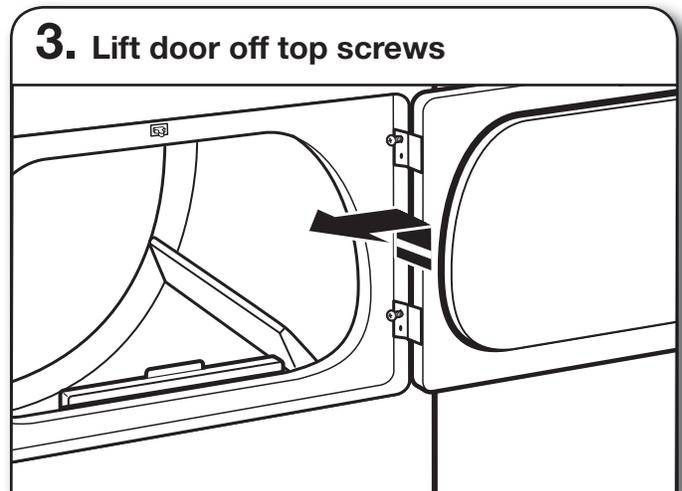
Lift door until top screws in dryer cabinet are in large part of hinge slot. Pull door forward off screws. Set door (handle side up) on top of dryer. Remove top screws from dryer cabinet.
