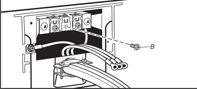
Remove center terminal block screw (B).
