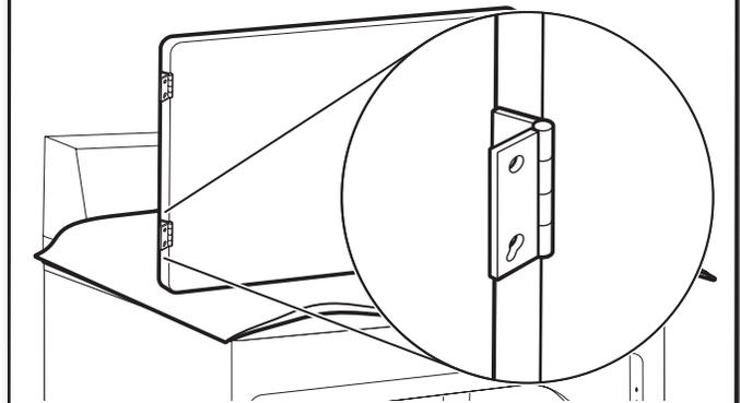
Reattach door hinges to dryer door so that the larger hole is at the bottom of the hinge.
