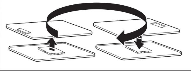
Rotate outer door 180° and set it back down on inner door. Be certain to keep cardboard spacer centered between doors. Reattach outer door panel to inner door panel so handle is on the side where hinges were just removed. Insert six door screws.
