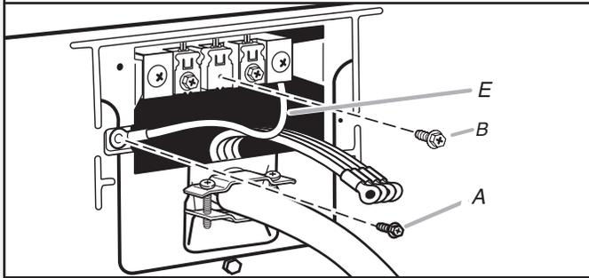
Remove center terminal block screw (B). Remove neutral ground wire (E) from external ground conductor screw (A).
