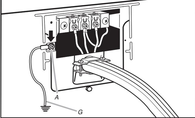
Connect a separate copper ground wire (G) from the external ground conductor screw (A) to an adequate ground. Finally, reinsert tab of terminal block cover into slot of dryer rear panel. Secure cover with hold-down screw. Now, go to "Venting Requirements."
