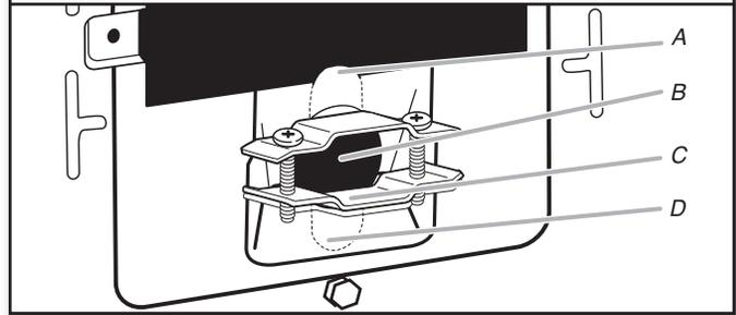
Remove the screws from a 3/4" (19 mm) UL Listed strain relief. Put the tabs of the two clamp sections (C) into the hole below the terminal block opening (B) so that one tab is pointing up (A) and the other is pointing down (D), and hold in place. Tighten strain relief screws just enough to hold the two clamp sections (C) together.
