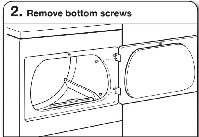
Open dryer door. Remove bottom screws from dryer cabinet side of hinges. Loosen (do not remove) top screws from dryer cabinet side of hinges.
