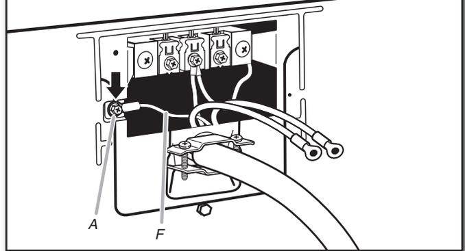
Connect ground wire (F) (green or bare) of power supply cord to external ground conductor screw (A). Tighten screw.
