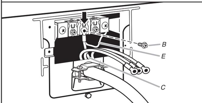
Connect neutral ground wire (E) and neutral wire (white or center) (C) of power supply cord under center terminal block screw (B). Tighten screw.
