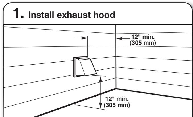
Install exhaust hood and use caulking compound to seal exterior wall opening around exhaust hood.
