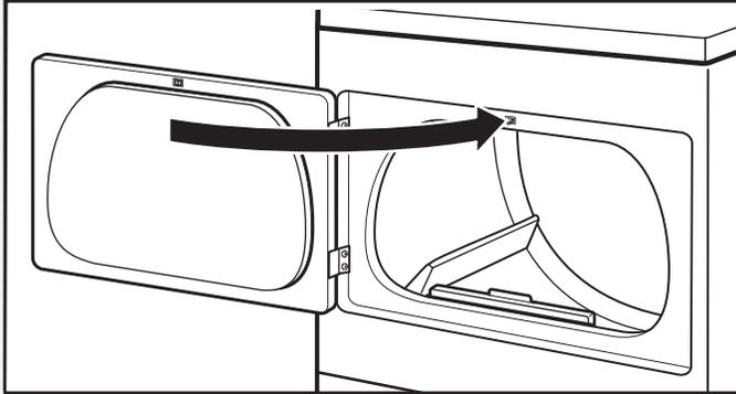
Close door and check that door strike aligns with door catch. If it is needed, slide door catch left or right within slot to adjust alignment.
