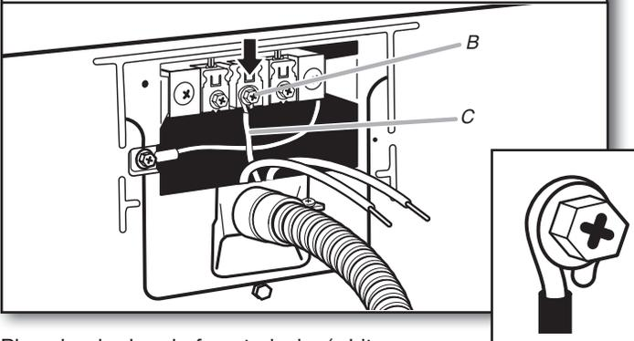
Place hooked end of neutral wire (white or center) (C) of direct wire cable under center terminal block screw (B). Squeeze hooked end together. Tighten screw.
