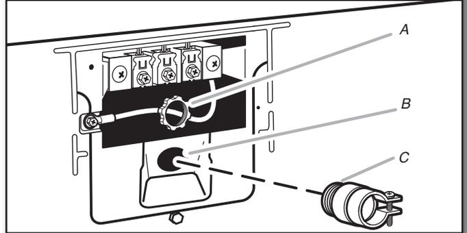
Unscrew the removable conduit connector (A) and any screws from a 3/4" (19 mm) UL Listed strain relief. Put the threaded section of the strain relief (C) through the hole below the terminal block opening (B). Reaching inside the terminal block opening, screw the removable conduit connector (A) onto the strain relief threads.
