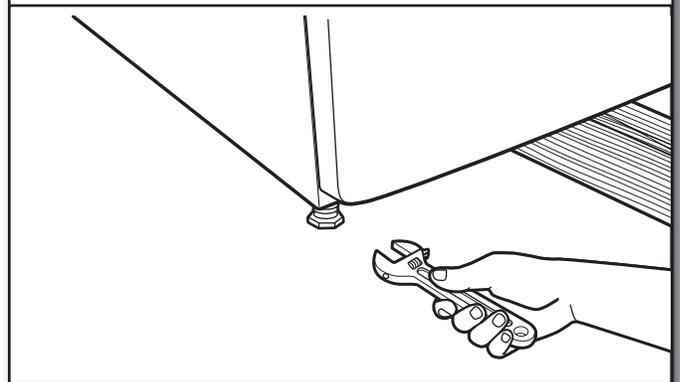
If dryer is not level, prop up using a wood block, use wrench to adjust legs up or down, and check again for levelness. Once dryer is level, make sure all four legs are snug against the floor before tightening them.
