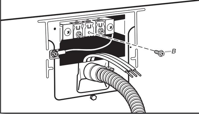
Remove center terminal block screw (B).
