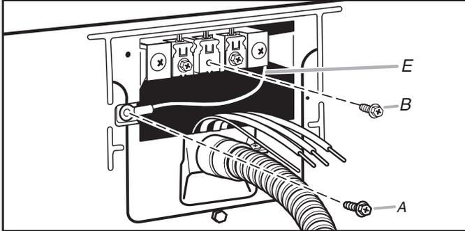
Remove center terminal block screw (B). Remove neutral ground wire (E) from external ground conductor screw (A).
