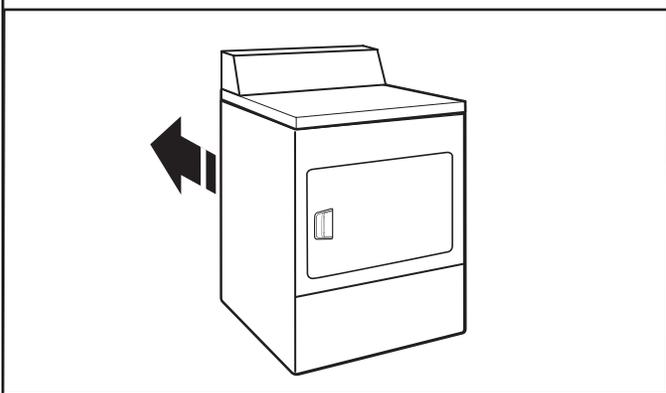
Move dryer to final location. Avoid crushing or kinking vent. After dryer is in place, remove corner posts and cardboard from under the dryer.
