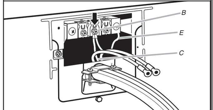
Connect neutral ground wire (E) and neutral wire (white or center wire) (C) of power supply cord or cable under center terminal block screw (B). Tighten screw.
