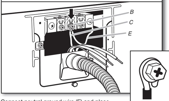
Connect neutral ground wire (E) and place hooked end (hook facing right) of neutral wire (white or center wire) (C) of direct wire cable under center screw of terminal block (B). Squeeze hooked ends together and tighten screw.
