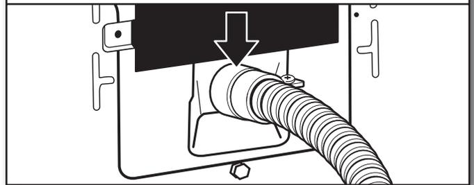
Put direct wire cable through the strain relief. The strain relief should have a tight fit with the dryer cabinet and be in a horizontal position. Tighten strain relief screw against the direct wire cable.
