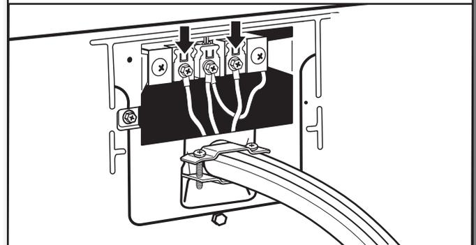
Place hooked ends of remaining wires under outer terminal block screws (hooks facing right). Tighten screws.
