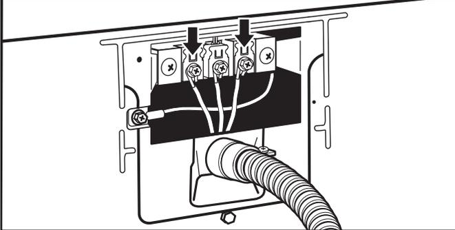
Place hooked ends of remaining direct wire cable wires under outer terminal block screws (hooks facing right). Squeeze hooked ends together and tighten screws. Finally, reinsert tab of terminal block cover into slot of dryer rear panel. Secure cover with hold-down screw. Now, go to "Venting Requirements."
