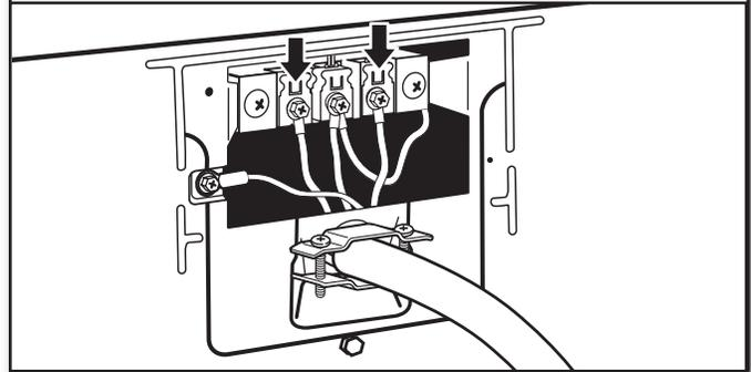
Connect remaining wires to outer terminal block screws. Tighten screws. Finally, reinsert tab of terminal block cover into slot of dryer rear panel. Secure cover with hold-down screw. Now, go to "Venting Requirements."
