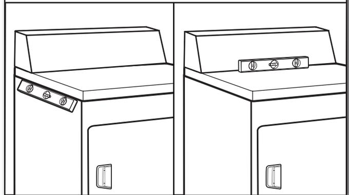
Check levelness of dryer from side to side. Repeat from front to back.
