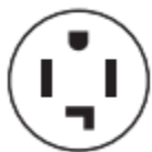
4-wire receptacle (14-30R)
