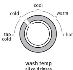
Once you select a cycle, select the desired wash temperature by turning the Wash Temp knob to the desired setting.
