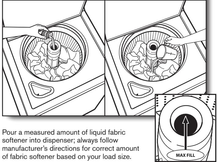
Pour a measured amount of liquid fabric softener into dispenser; always follow manufacturer's directions for correct amount of fabric softener based on your load size.
