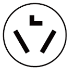
3-Wire receptacle (10-30R)
