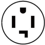
4-Wire receptacle (14-30R)
