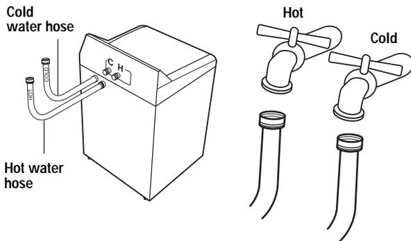
5. Tighten each connection by hand, then tighten another 2/3 turn with pliers. Do not cross-thread or over-tighten these connections.
