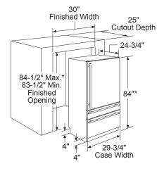
\* 84" High installation. The refrigerator can be adjusted to fit into a cutout that is 83-1/2" min. to 84-1/2" max with the appropriate door kit. Use leveling legs and wheels for a maximum 1" height adjustment.
