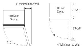
**NOTE:** Clearances are based on the recommended 2-1/4" handle standoff depth.
