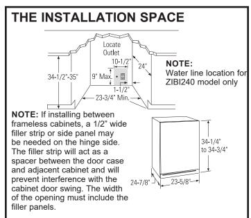
The product must be installed so that the custom panel front will project 2-3/4" forward of adjacent cabinets. This position will allow a full door swing and prevent interference with adjacent cabinetry. The opening between cabinets must be 23-3/4" minimum. These models can not be installed flush in 24"-deep cabinets.
