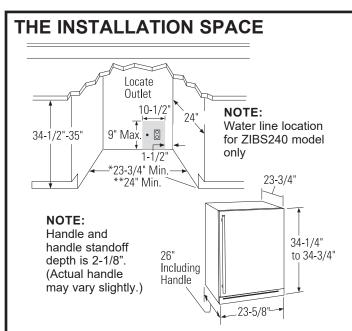
\*For a standard installation: The product must be installed so that the stainless steel front will project 1-5/8" forward of adjacent cabinets. This position will allow a full door swing and prevent interference with adjacent cabinetry. The opening between cabinets must be 23-3/4" minimum.
