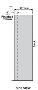
FLUSH 3/4" THICK PANEL DIMENSIONS SINGLE INSTALLATION
