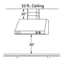
**10 ft. ceilings:** When the hood is installed 36" above the cooking surface, order three 12" and one 6" duct cover accessories.
