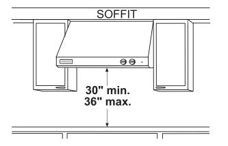
In this installation the ductwork running from the top of the hood will be concealed in the soffit or upper cabinetry.
