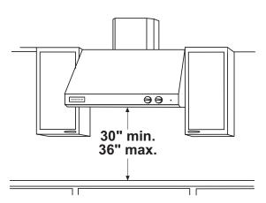
For this installation, a decorative duct cover is available to conceal the ductwork running from the top of the hood. Use of the duct cover requires special consideration to the installation height above the countertop.
