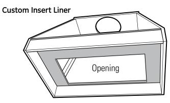
The custom canopy must be sized to fit the insert sleeve. Construct the canopy with an opening that is: 38-3/4"W  $\times$  13-3/16"D
