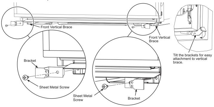
■ Attach the BOTTOM TRIM to these brackets with the flange inside the cabinet and toward the bottom. Use machine screws provided.
