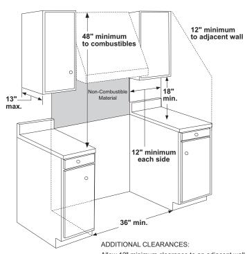
Allow 12" minimum clearance to an adjacent wall on each side.
