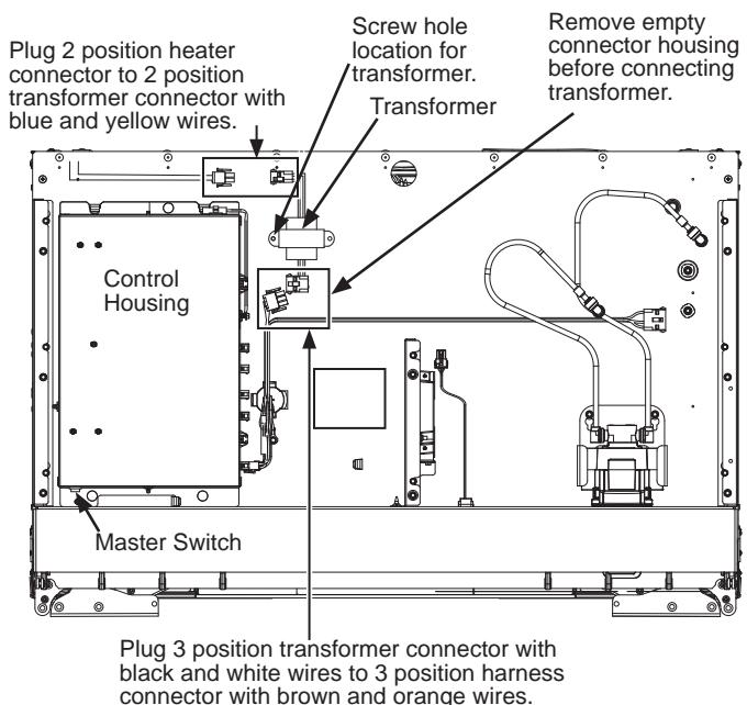
Plug 2 position heater connector to 2 position transformer connector with blue and yellow wires.
