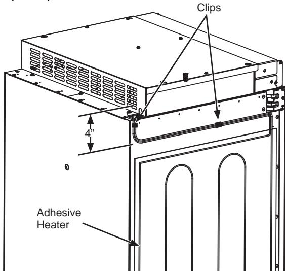
**NOTE:** The heater installation is available only on the left side of compatible models.
