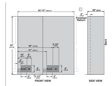
DUAL INSTALLATION 36" INTEGRATED FREEZER, ZIF361NBRII AND 36" INTEGRATED REFIGERATOR, ZIR361NBRII
