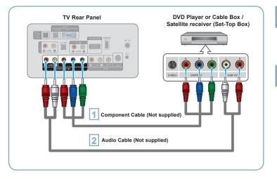
Connect a Component Cable between the COMPONENT IN [Y,  $P_B$ ,  $P_R$ ] jacks on the TV and the COMPONENT [Y,  $P_B$ ,  $P_R$ ] jacks on the DVD Player or Cable Box/Satellite receiver (Set-Top Box).
