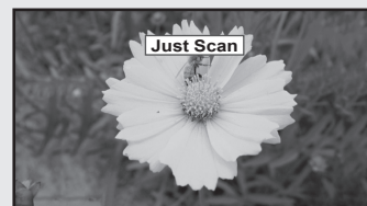
Just Scan Use the function to see the full image without any cutoff when HDMI (720p/1080i/1080p), Component (1080i/1080p) or DTV (1080i) signals are input.
